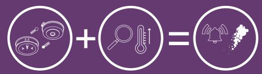
Data sent between dual sensors monitoring heat and smoke levels If a rise in temperature is detected by the heat sensor... ...data will relay to the optical sensor, increasing it's sensitivity to smoke
